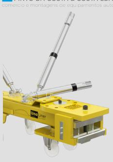
The UnoLiner P20 Vector Pulling set is a 10 metric ton hydraulic cylinder connected to an air operated hydraulic high pressure pump and in combination with the chain holder, Lock Pin and Vector Pulling extension tubes is mounted on the UnoLiner P10 Pulling Tower enabling multi-directional pulls in combination with the optional D10 Down Pull Adapter.
