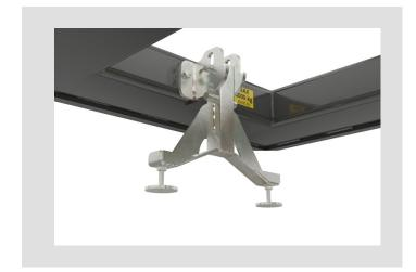
UnoLiner F1030 Bench Height Set to set the bench at the correct height for connecting the UnoLiner P10 Draw Aligner Pulling Tower to the Straightening Bench. The P10 Pulling Tower rolls straight and easily into position at the correct bench height and is locked onto the bench with the tightening of **One Bolt**.
