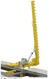
With the P3030 Pull Arm Extension fitted to the P10 Pulling Tower, the height, range and angle of any pull can be extended by 87 cm enabling a greater range and distance for pulling from a chosen location on the UnoLiner chassis straightening bench frame.
